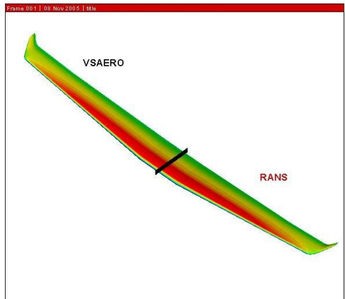
Fig 1-wing+winglet; Identical superficial mesh 10 800 panels
