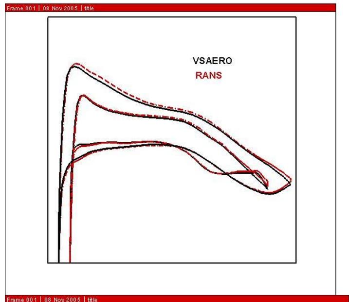
Fig.2 Distribution of pressure along the wing cords
