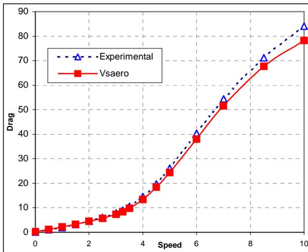
Figure 2. Drag vs. Speed for an America's cup Yacht in the downwind condition.
