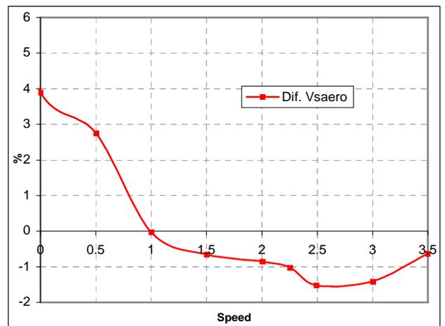
Figure 5. % error in drag vs. speed for the upwind case
