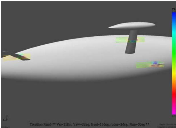
Figure 9. Off-body streamlines on the rudder, daggerboard and Keel, with off-body velocity visualisation.
