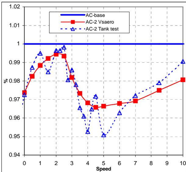
Figure 6 Percentage difference in drag on two different Americas Cup yachts calculated with VSAERO and tested in a towing tank.
