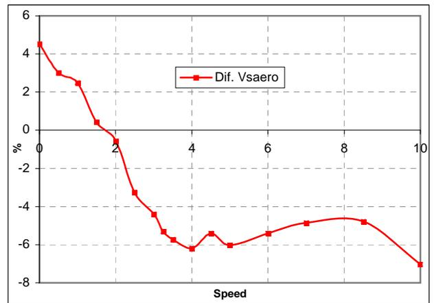
Figure 4. % error in drag vs. speed for the downwind case
