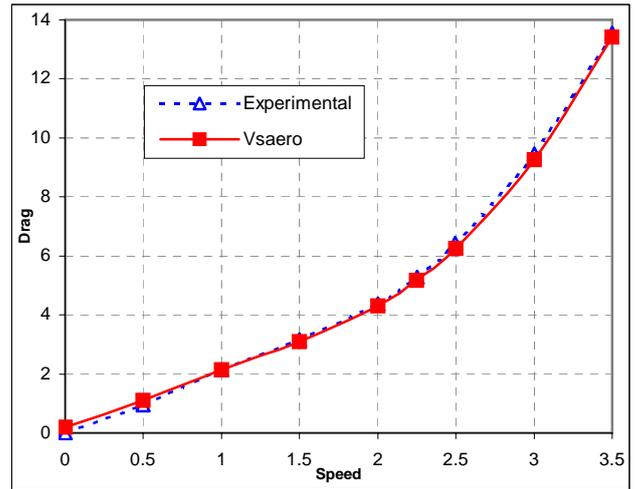
Figure 3. Drag vs. Speed for an America's Cup yacht in an upwind condition
