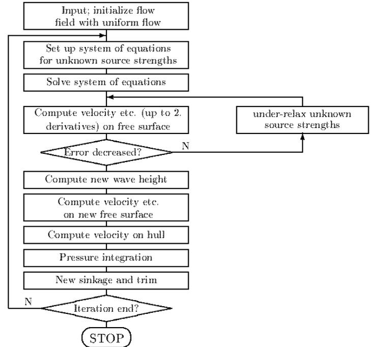
Figure 1. Flow chart of the iterative solution.
