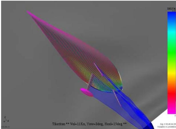
Figure 8. On-body streamlines with boundary layer thickness and wake visualisation.
